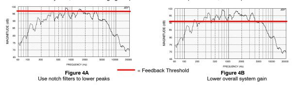
FREQUENCY RESPONSE OF AN UNEQUALIZED SOUND SYSTEM Figure 4
